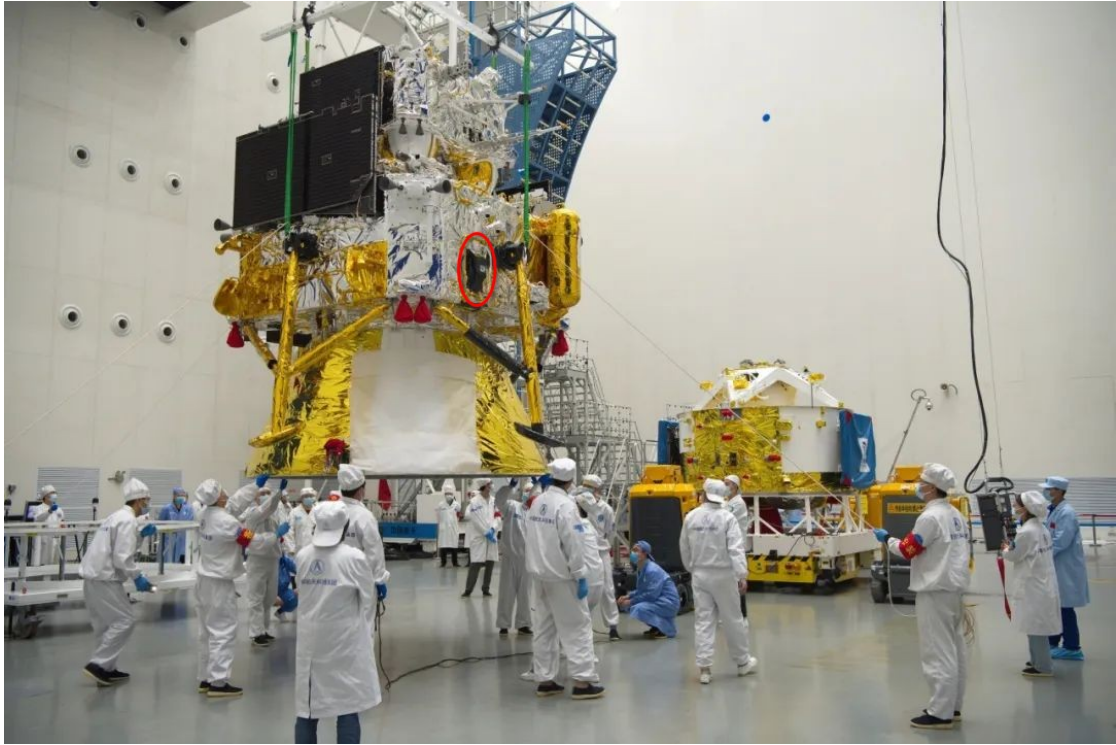
Figure 1.1: Assembly of Chang'E-6 spacecraft. On the left side, from top to bottom, there is the ascender, the lander and the returner. On the right side there is the orbiter. The NILS instrument (red circle) is mounted on the lander. Image credit: CNSA/CLEP.
